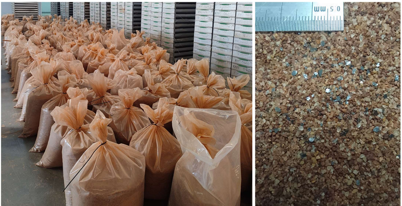
Figures 3 & 4: LHS: Four tonne graphite pre-concentrate sample produced at the Company's Lilongwe laboratory RHS: Close-up of the pre-concentrate showing the coarse, clean graphite flakes
