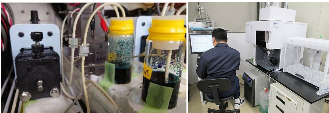
Figure 2: Mini-cell testing of TMT vanadium electrolyte – LE System's Tsukuba Technical Centre, in Ibaraki, Japan.
