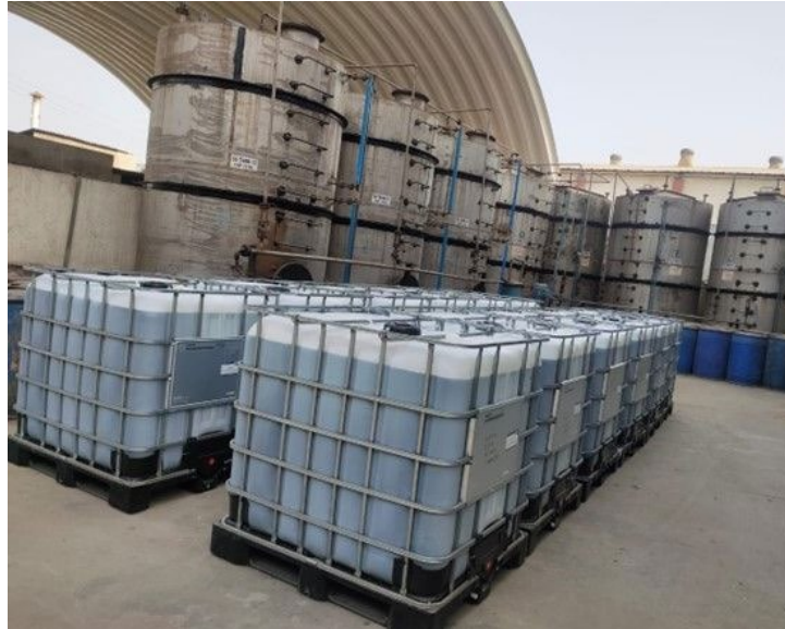
Figure 1: Delectrik vanadium electrolyte ready for export
