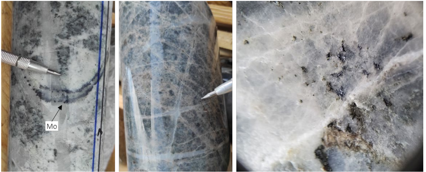
Plate 2. Left: CRDD22-001 (494m) Diorite porphyry with phyllic alteration, 1-2% disseminated chalcopyrite, 2-3% pyrite, 1-2% molybdenite in B-type quartz vein, intensive > 5% quartz veinlet stockwork. Middle: CRDD22-001 (530m) Andesite with potassic alteration, 2-3% disseminated pyrite, trace < 1% chalcopyrite, trace < 1% molybdenite, intensive > 5% quartz veinlet stockwork. Right: CRDD22-002 (94m) Diorite Porphyry with phyllic alteration, 0.5-1% disseminated chalcopyrite, 2-3% pyrite, 0.5-1% molybdenite in B-type veins.
