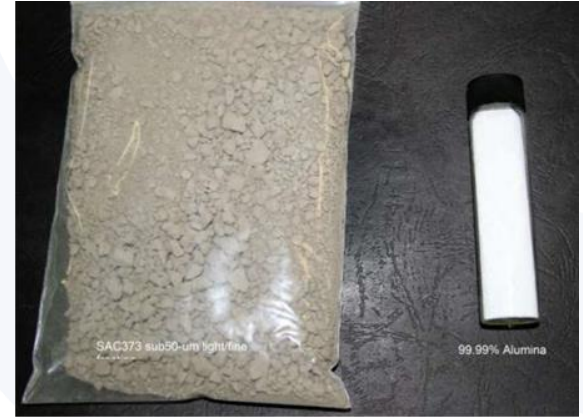
Above: Saprolitic clay from SAC373 used to produce HPA via testwork by Salazar Gold
