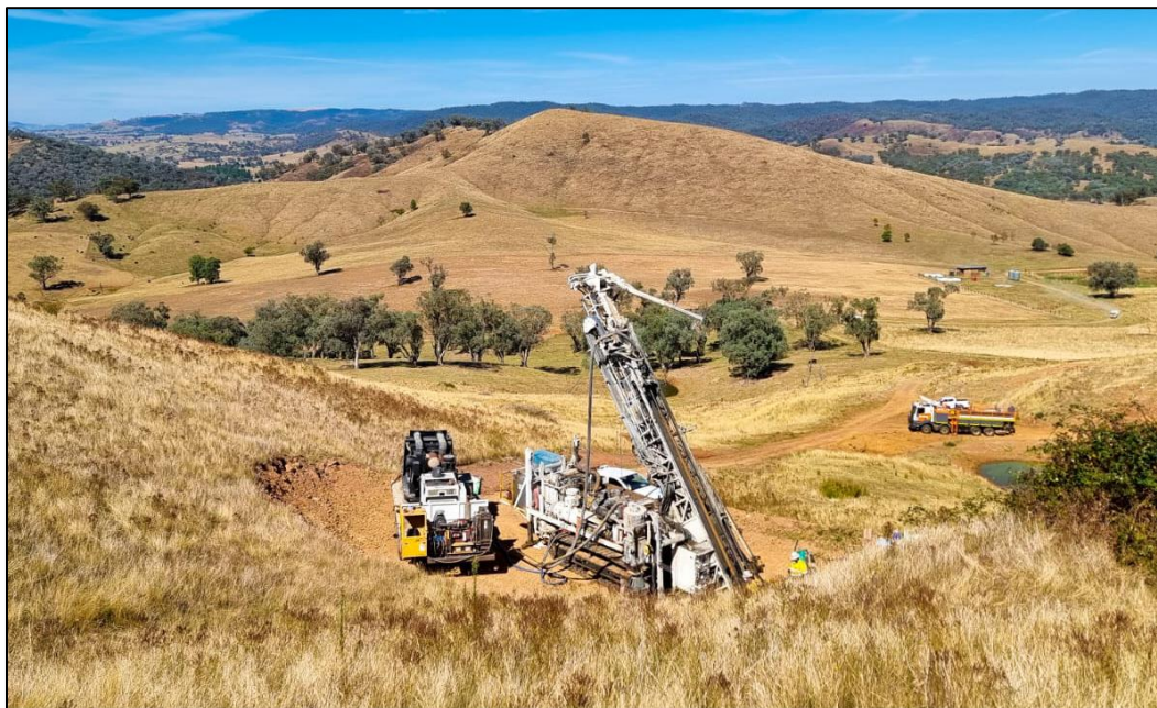
Figure 1 – Durock Drilling’s track-mounted RC rig drilled 1,713m, completing the Phase 2 drilling of the Greater Hobbs Pipe area at the Mt Adrah Project, Lachlan Fold, NSW.
