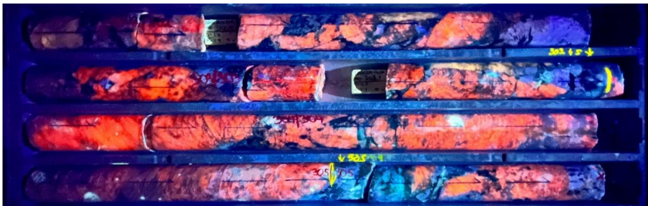
Figure 1 – TARC161D diamond core from 301.8m to 305.5m from the Leia Pegmatite under ultraviolet light suggesting ~70% coarse spodumene (salmon orange) ~30% feldspar, quartz and muscovite (blue/grey)
