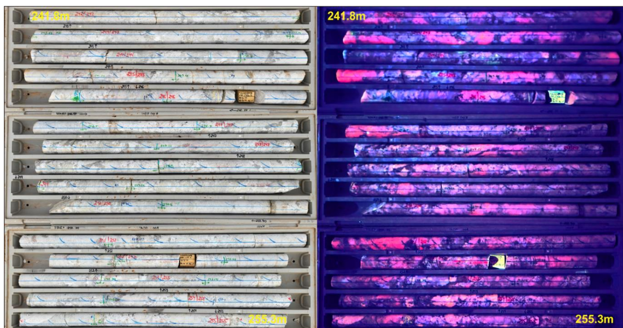
Figure 2: Core from TADD008 under natural and fluorescent light indicating abundant spodumene comprising up to 50% of the core, which typically fluoresces bright salmon orange under UV light. Note that assays for this hole are pending.
