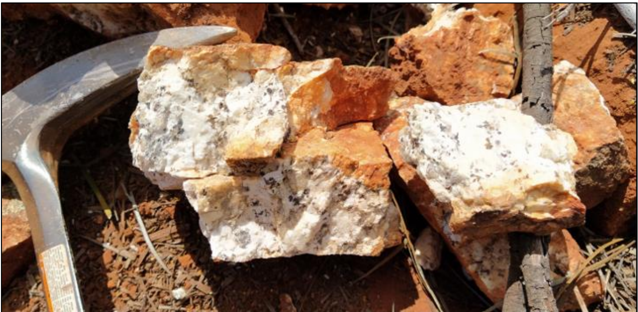
Figure 3 – Plagioclase and perthitic textured quartz pegmatite with possible disseminated tantalite (302,005mE, 6,577,381mN) 2
