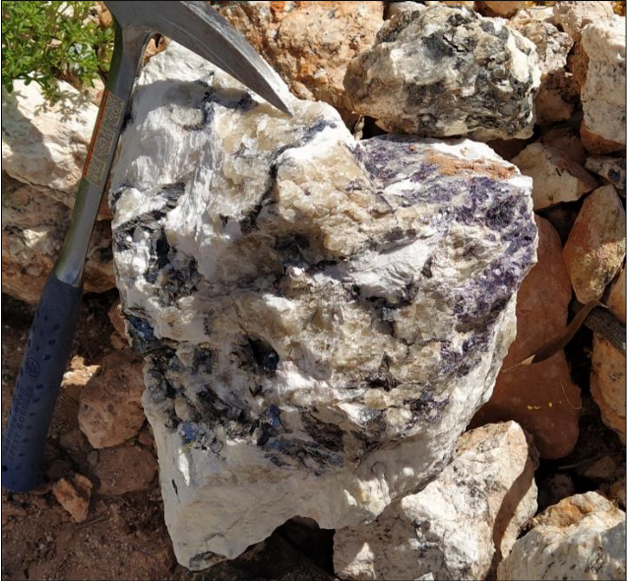
Figure 2 – Lepidolite, zinnwaldite, plagioclase, quartz pegmatite from the Red Panda costean (301,792mE, 6,577,339mN) 2
