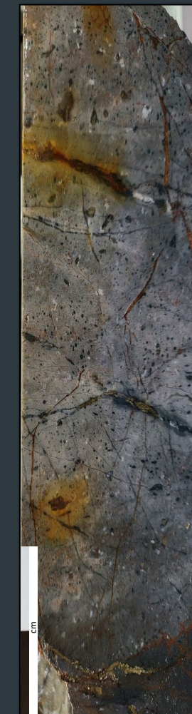
K-spar + albite + silica + tourmaline alteration, 2g/t Au, 0.14% Cu (Alkalic lithocap porphyry alteration, SD010 – 196m)
