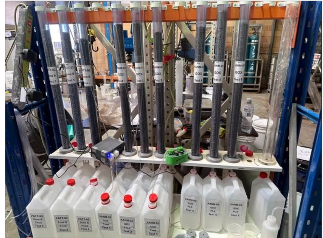
Oxide Column Leach at Draslovka Mining Process Solutions Labs
