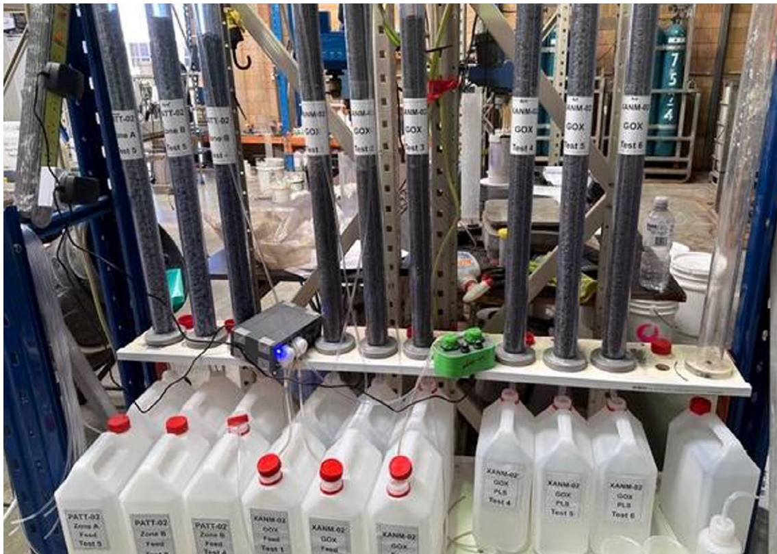
Figure 4: Oxide Column Leach at Draslovka Mining Process Solutions
